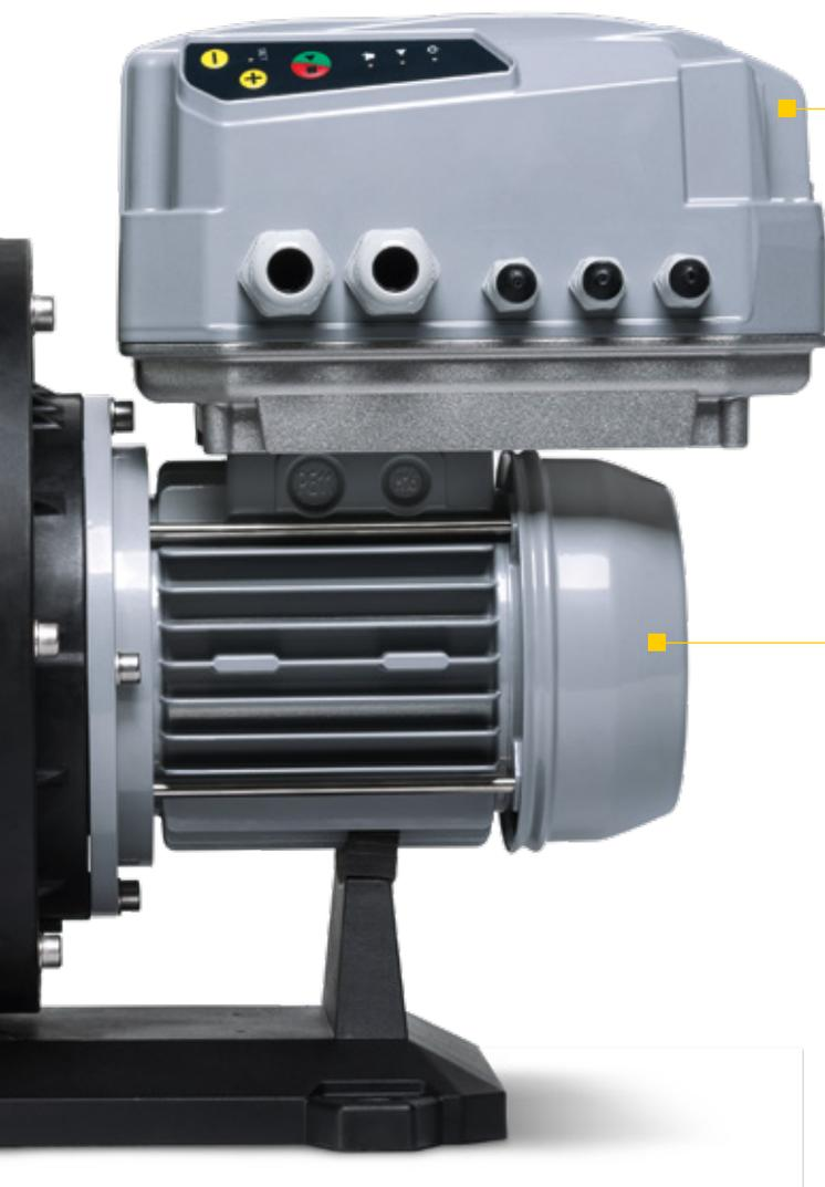
■ **Integrated inverter** attached to the motor, exclusively in aluminium, and with independent ventilation to guarantee excellent thermal performance.
